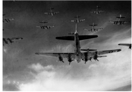
PHOTO: A mass of B-17 bombers, flying in a 'box' formation that allowed their defensive guns to provide mutual support.
