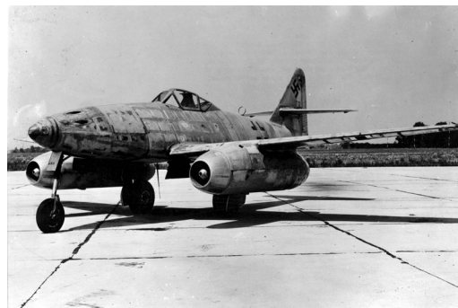
PHOTO: Jets were an immature technology, and in the case of the Me 262 it was rushed into service with unreliable, short lifespan engines. Though it showed potential, the Allies found ways to keep the jet threat suppressed.
